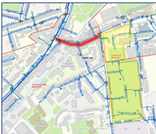
Figure 5.1 - Section of Watermain Requiring Upgrade
